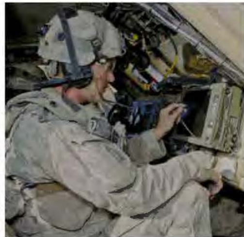
Figure 1-6. Commander using a JBC-P JV5 Block 2 on a Multi-Domain Atlas display
