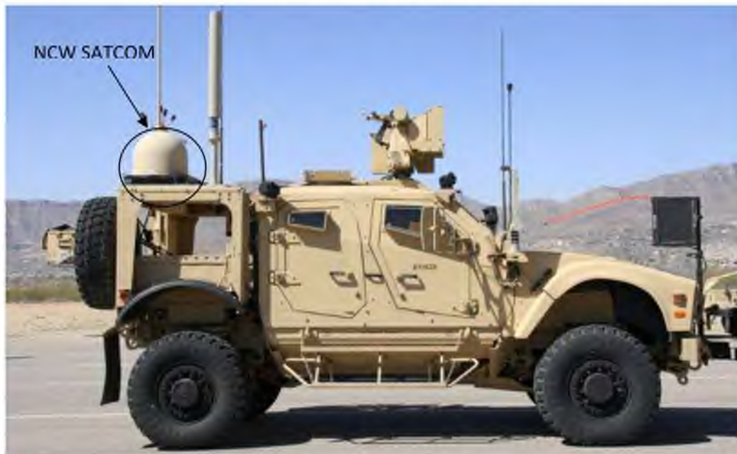
Figure 1-3. WIN-T Increment 2 SNE, Installed in an M-ATV
