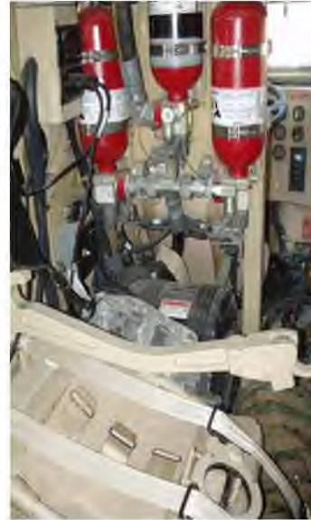
Figure 5-3. FPI Cougar Ambulance Fire Extinguishing Valves and Litter Interference
