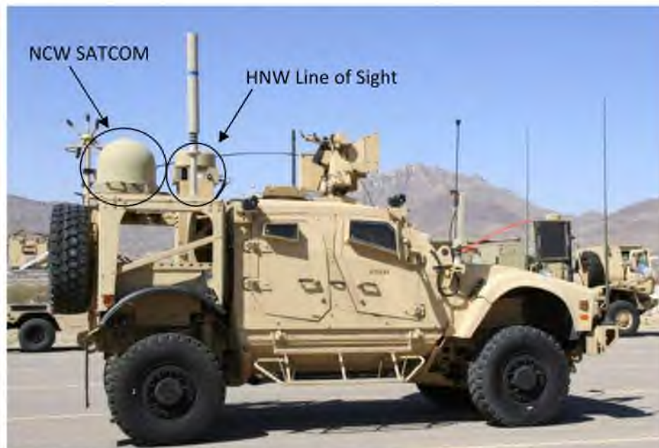
Figure 1-2. WIN-T Increment 2 PoP, Installed in an MRAP All-Terrain Vehicle (M-ATV)
