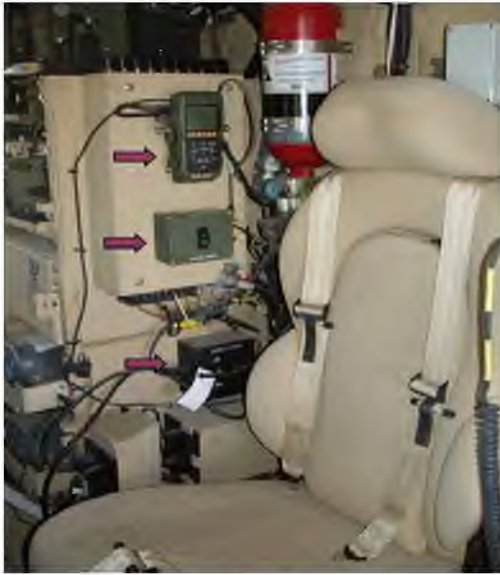
Figure 5-2. FPI Cougar Ambulance Medical Attendant Seat; Command and Control Switch Interference
