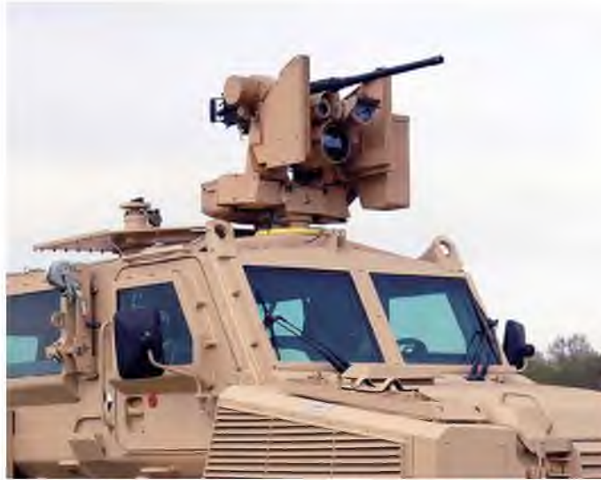
CROWS with an M2 machine gun mounted on a Mine Resistant Ambush Protected vehicle
