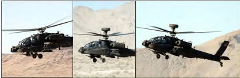
Figure 1. AB3 Configurations: Slick, with Data Link Antenna, and with Fire Control Radar
