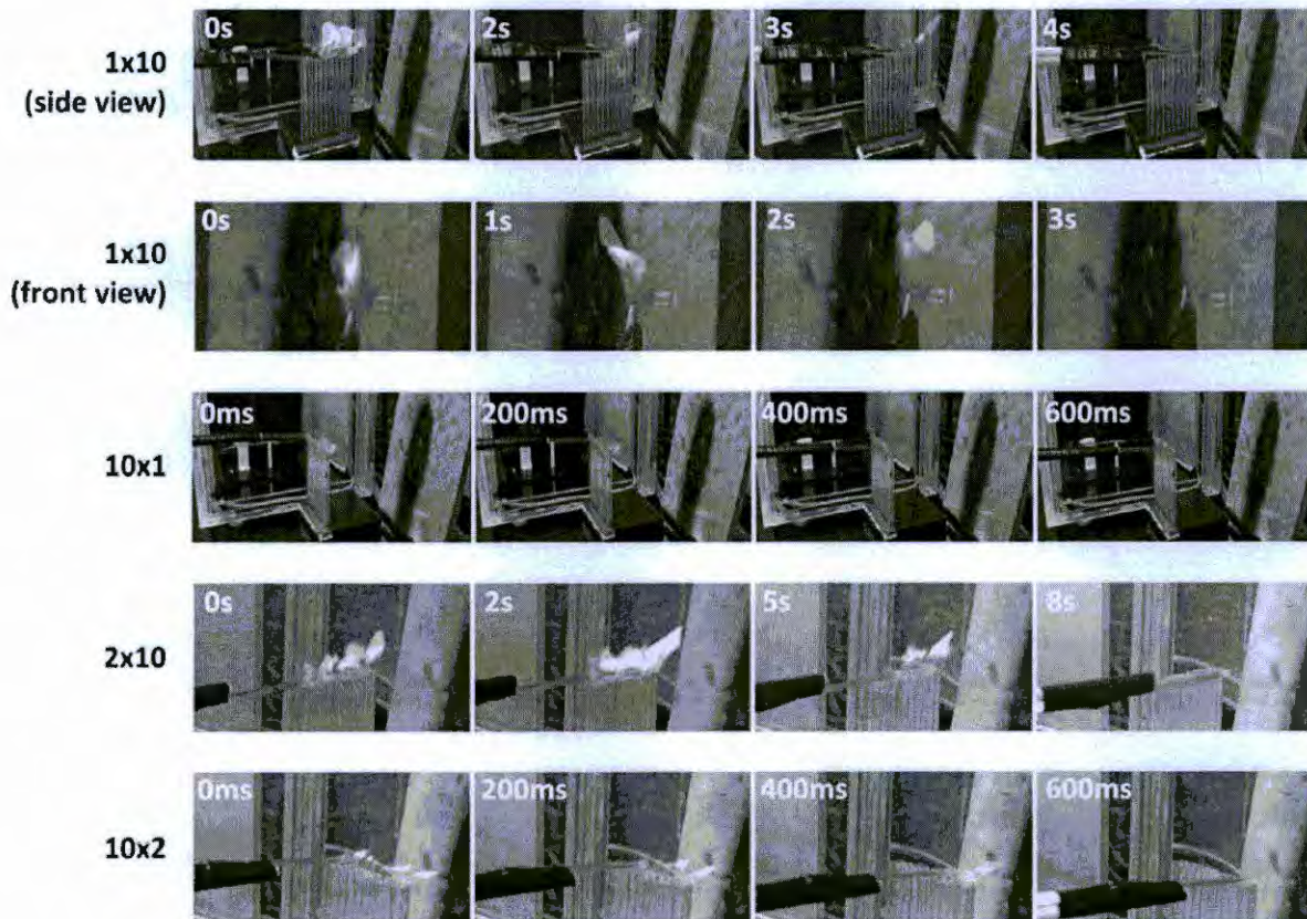
Figure 11. Snapshot of methane/air non-premixed flames generated by burner arrays and suppressed by a hand-held electrode raised to an AC potential of 40kV and 1.2 kHz.
