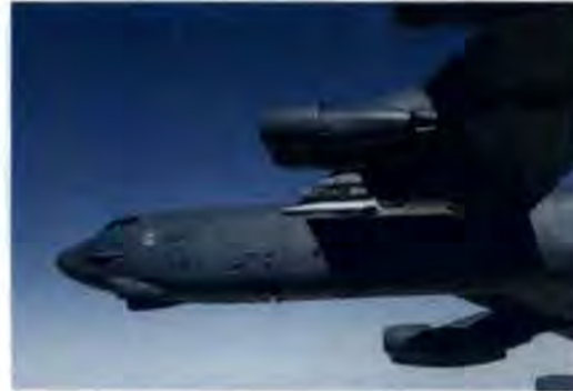
The X-51A Waverider prepares to launch its historic fourth and final flight. The cruiser achieved Mach 5.1 traveling 230 nautical miles in just over six minutes, making this test the longest air-breathing hypersonic flight ever. (U.S. Air Force photo/Bobbi Zapka)
