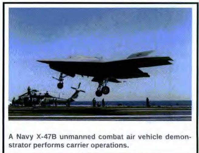
A Navy X-47B unmanned combat air vehicle demonstrator performs carrier operations.
