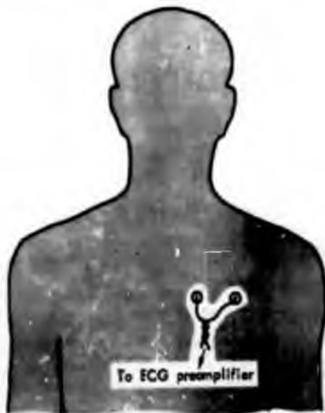
FIGURE 2. PLACEMENT OF ELECTRODES USED TO PICK UP THE HEART SIGNAL FOR TELEMETRY
