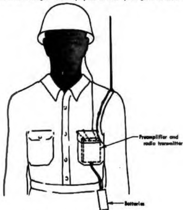
FIGURE 3. A GUARD WEARING THE BIOSIGNAL TELEMETRY EQUIPMENT
