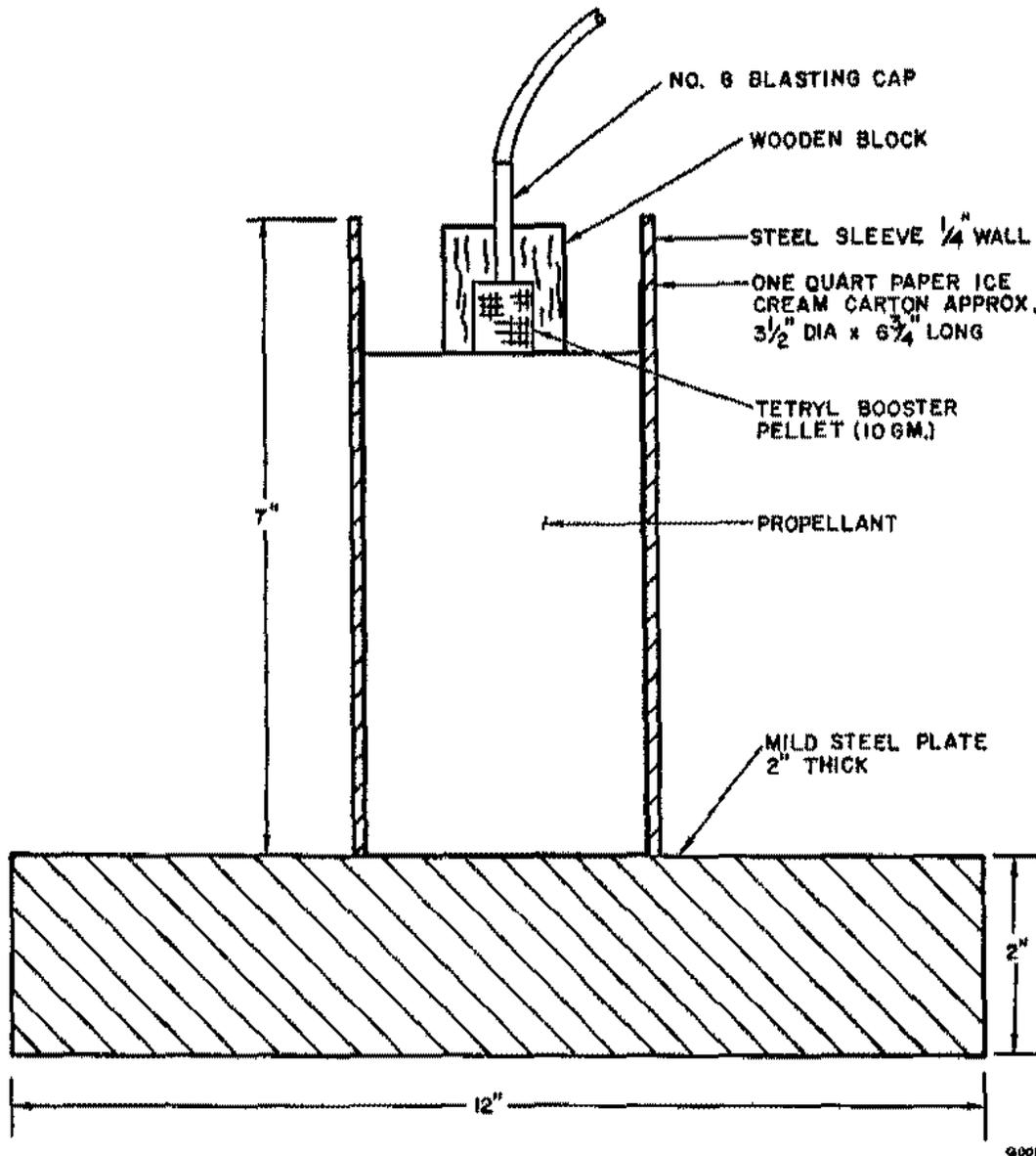
Figure 1. Section View of Field Explosive Test Setup for Susceptibility to Detonation Tests.
