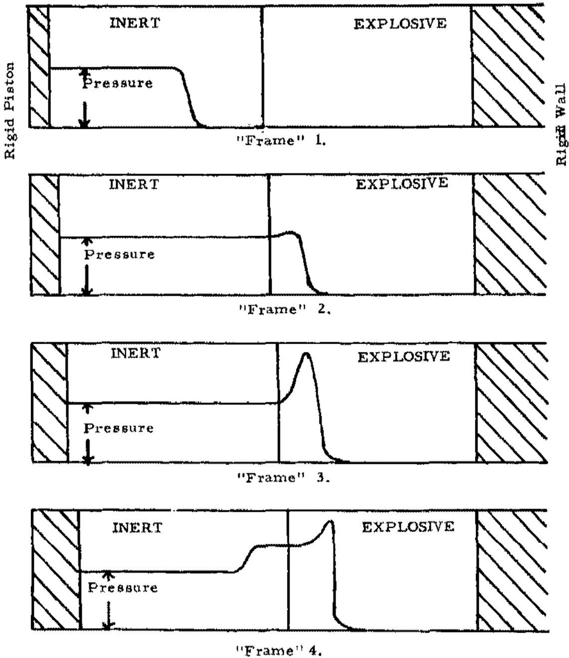
FIGURE 7. One Dimensional Theoretical Model for Gap Test. Inert Gap and explosive have the same equation of state. Progress of shock as a function of time. Piston moves at constant Velocity.
