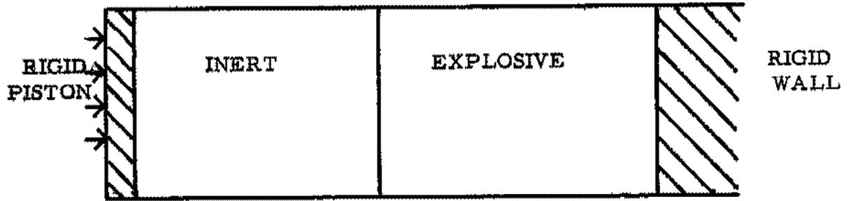
FIGURE 6. One Dimensional Model For Theoretical Treatment of Gap Test. Rigid Piston at Left Compresses Inert Material and Explosive Against Rigid Wall at Right.
