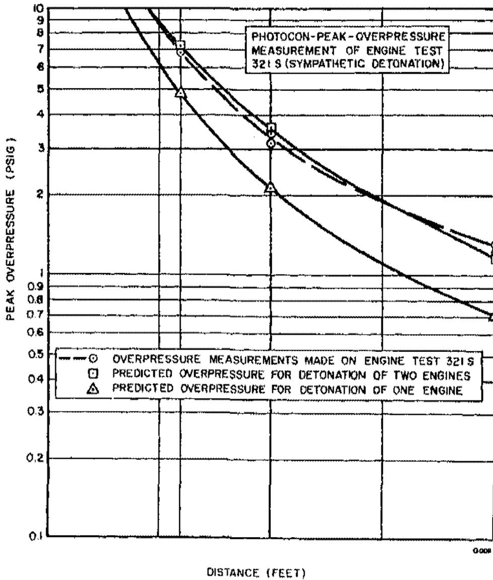
Figure 8. Test-Peak-Overpressure Measurement Versus Distance Superimposed on TNT Equivalence Plot Assuming 1.5 Reflection Coefficient.
