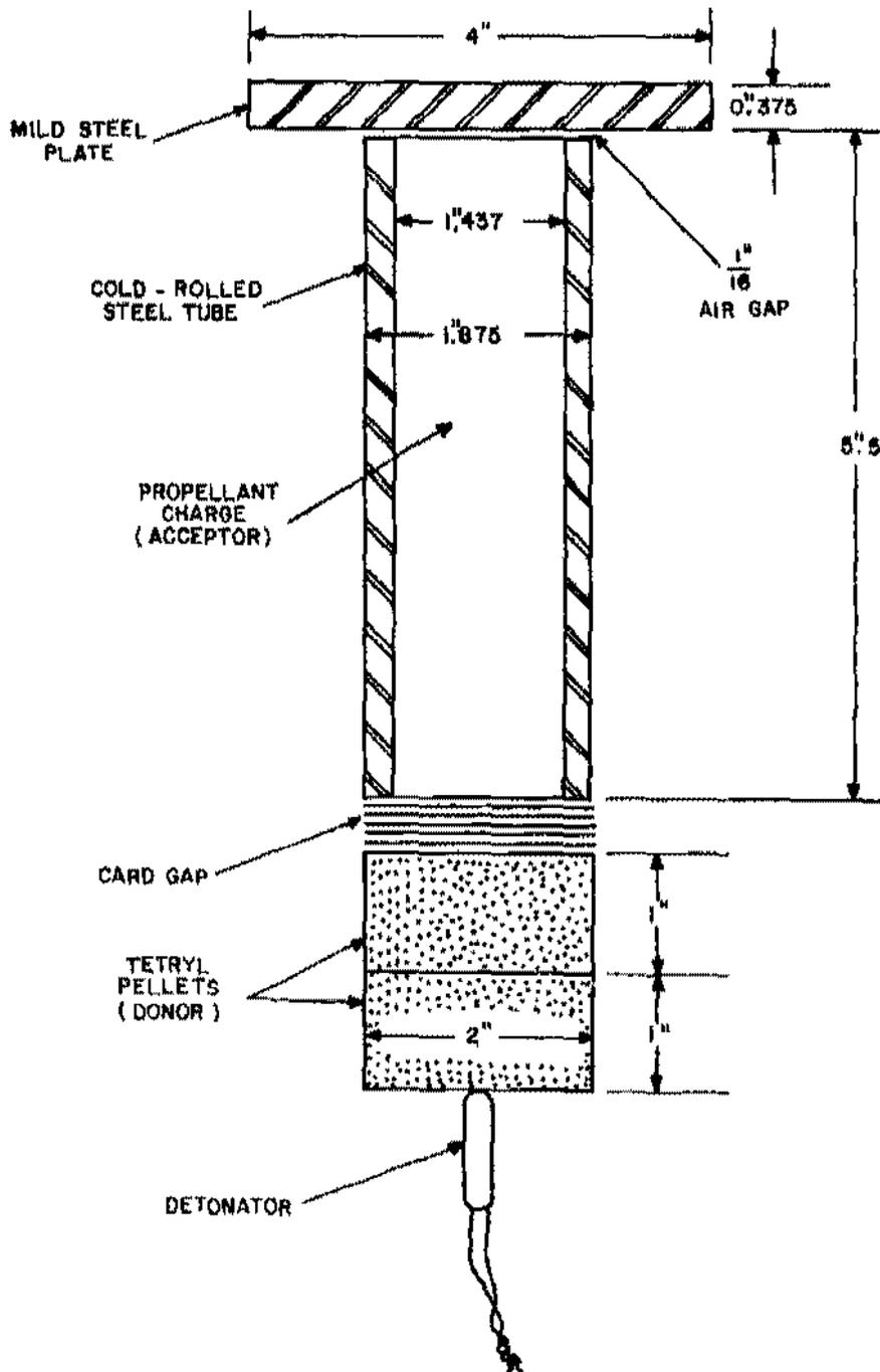
FIGURE 1. Gap Test for Solid Propellants
