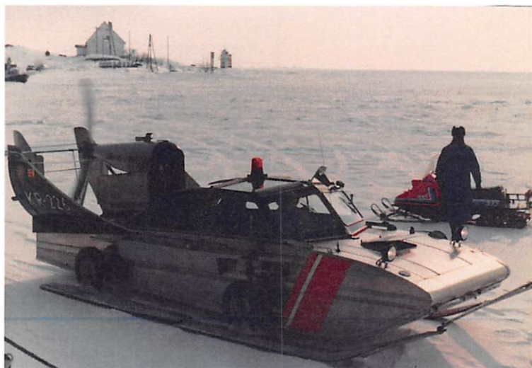
Figure 54: The ice-boat provide a flexible way to get around the Finnish coast during the winter. Note that in addition to being a boat, the vehicle has skis for the ice and wheels for land surfaces.
