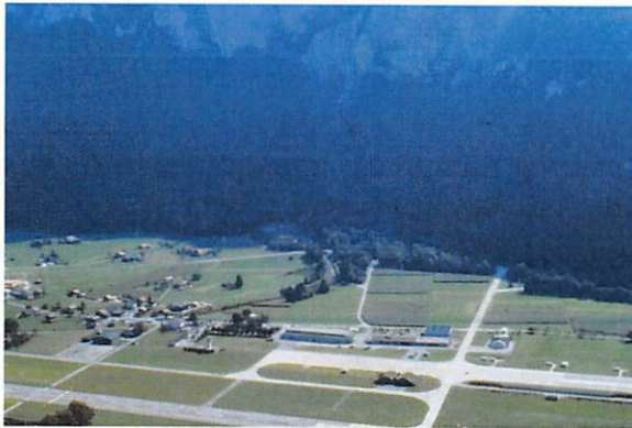
Figure 48: Note from the photograph at the left how the Norwegians managed to “mask” the entrances to the aircraft shelters and maintenance areas constructed into the mountains. Taxiways went behind “cover” before entering into the mountain so that the tunnel entrances themselves would be difficult to target.
