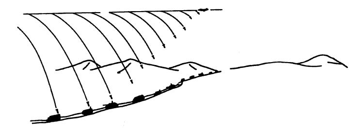
Figure F-6. Dispersion Pattern of Submunitions by Boost/Glide Vehicles, Cruise Missiles and Strike RPV's (U)
