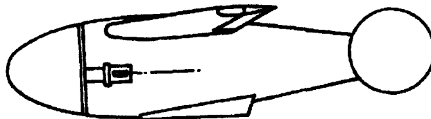
FIG. 6b Orientation of Pitch Gyro
