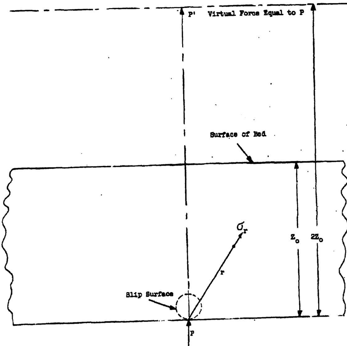
FIGURE 4.1.3 POINT LOAD IN A TWO DIMENSIONAL BED OF POWDER WITH A VIRTUAL FORCE TO CORRECT FOR BOUNDARY CONDITIONS ON THE SURFACE OF THE BED
