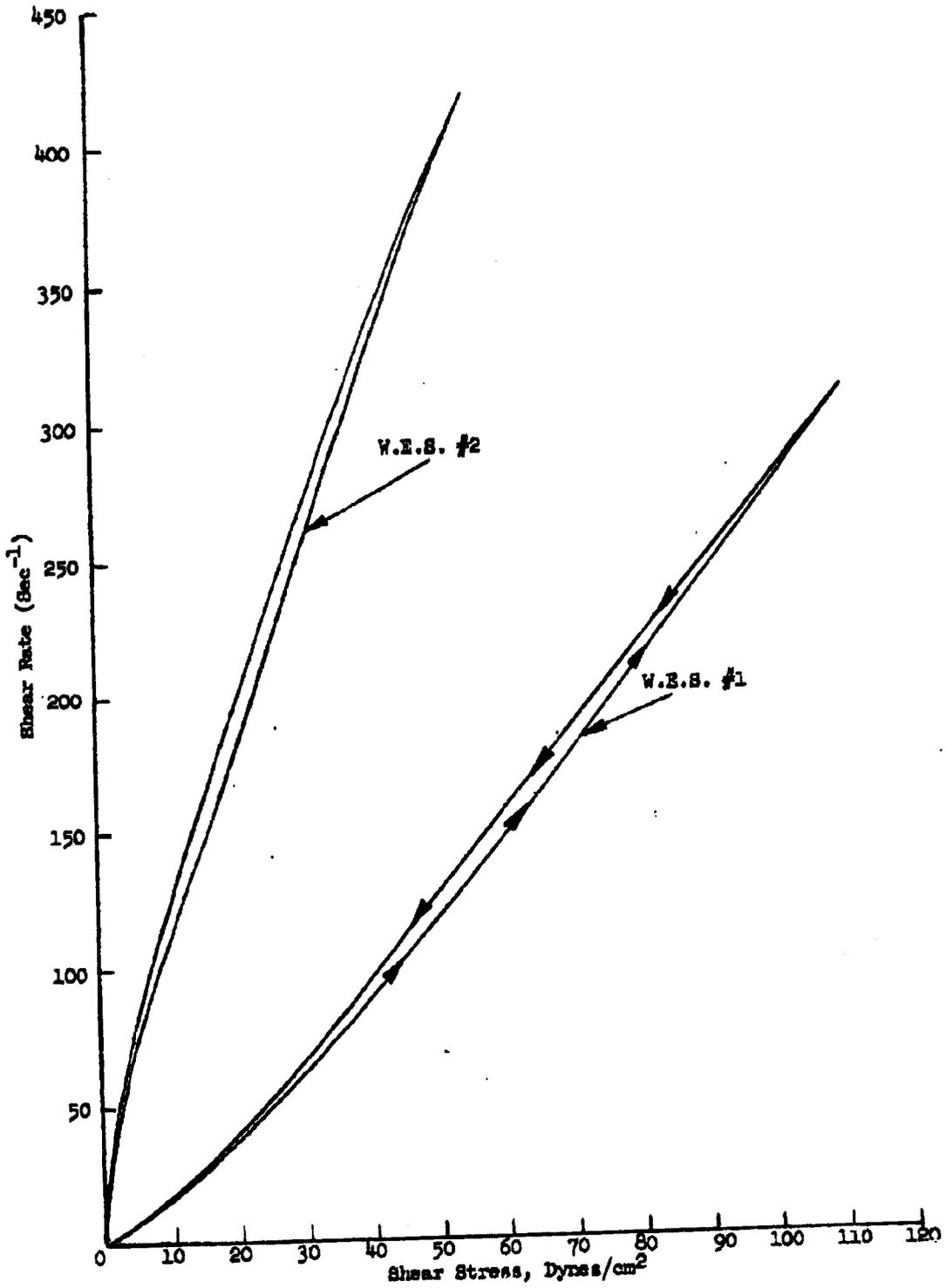
FIGURE 5.1.1 CONSISTENCY CURVES FOR W.E.B. #1 AND #2 AT 20°C
