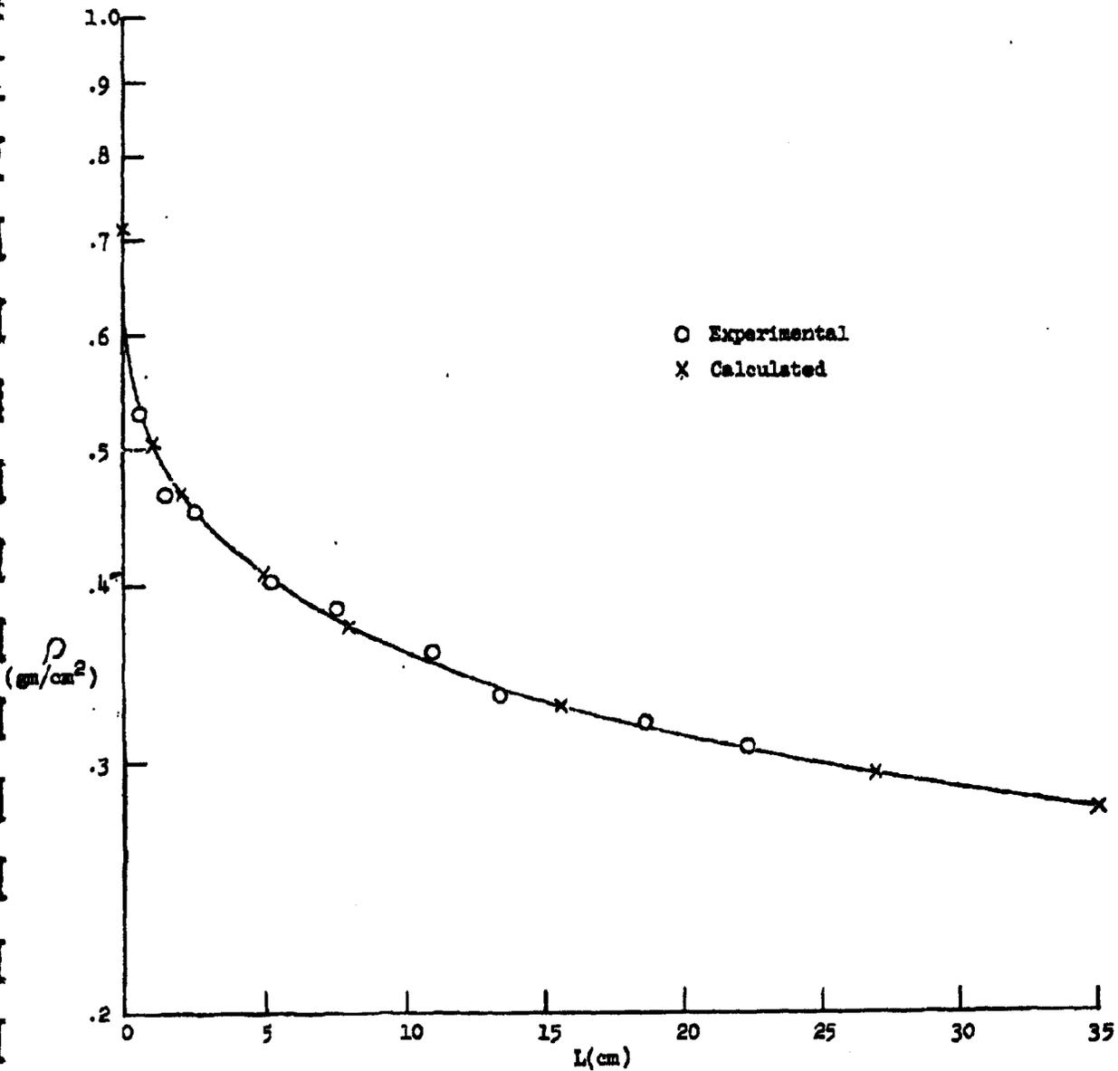
FIGURE 3.3.1 AVERAGE BULK DENSITY ( $\rho$ ) OF TALC AS A FUNCTION OF
