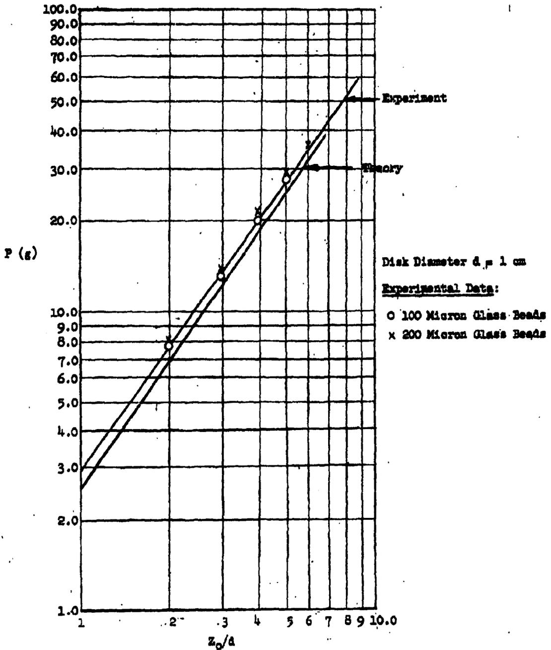
FIGURE 4.3.1 FORCE REQUIRED TO LIFT AN IMMERSED DISK FROM GRANULAR BED vs  $Z_0/d$
