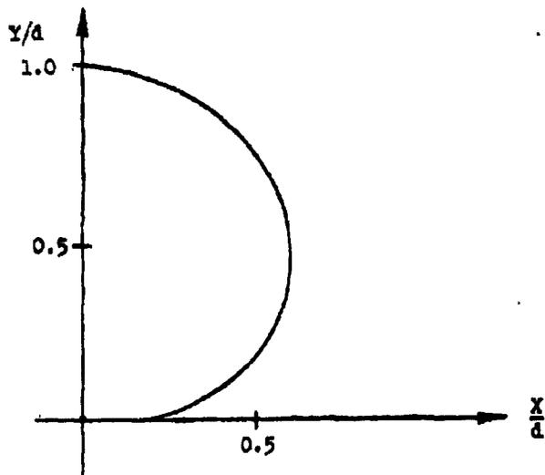
FIGURE 4.1.2 THEORETICAL TWO-DIMENSIONAL SLIP SURFACE;  $\phi = 30^\circ$ ,  $P/\pi/a^2 = 5$
