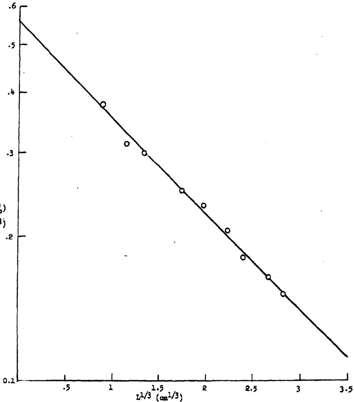
FIGURE 3.3.2 A PLOT OF  $(\rho - \rho_0)$  VS  $L^{1/3}$  FOR TALC UNDER A COMPRESSIVE FORCE OF  $3.72 \times 10^5$  Dynes/cm<sup>2</sup>
