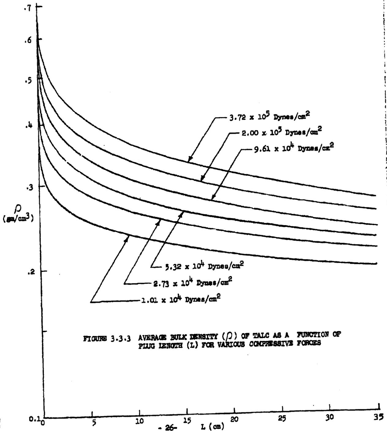
FIGURE 3.3.3 AVERAGE BULK DENSITY ( $\rho$ ) OF TALC AS A FUNCTION OF PLUG LENGTH ( $L$ ) FOR VARIOUS COMPRESSIVE FORCES
