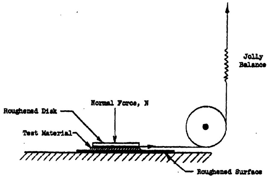
FIGURE 4.3.2 DIRECT SHEAR TEST APPARATUS
