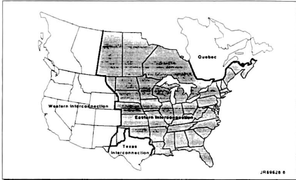
Figure 1: Interconnections of Utility Systems
