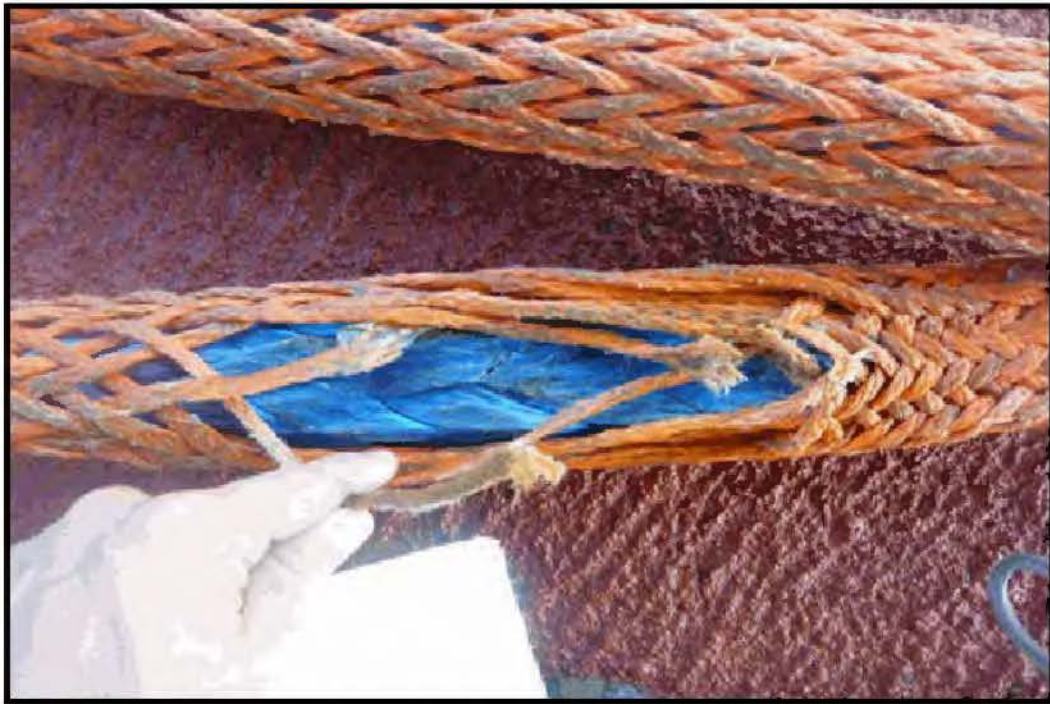
Figure 4-3. Mooring Line Damage
