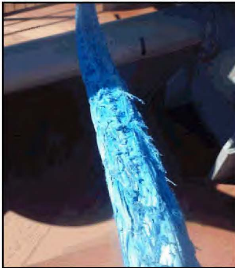
Figure 4-2. Mooring Line Damage
