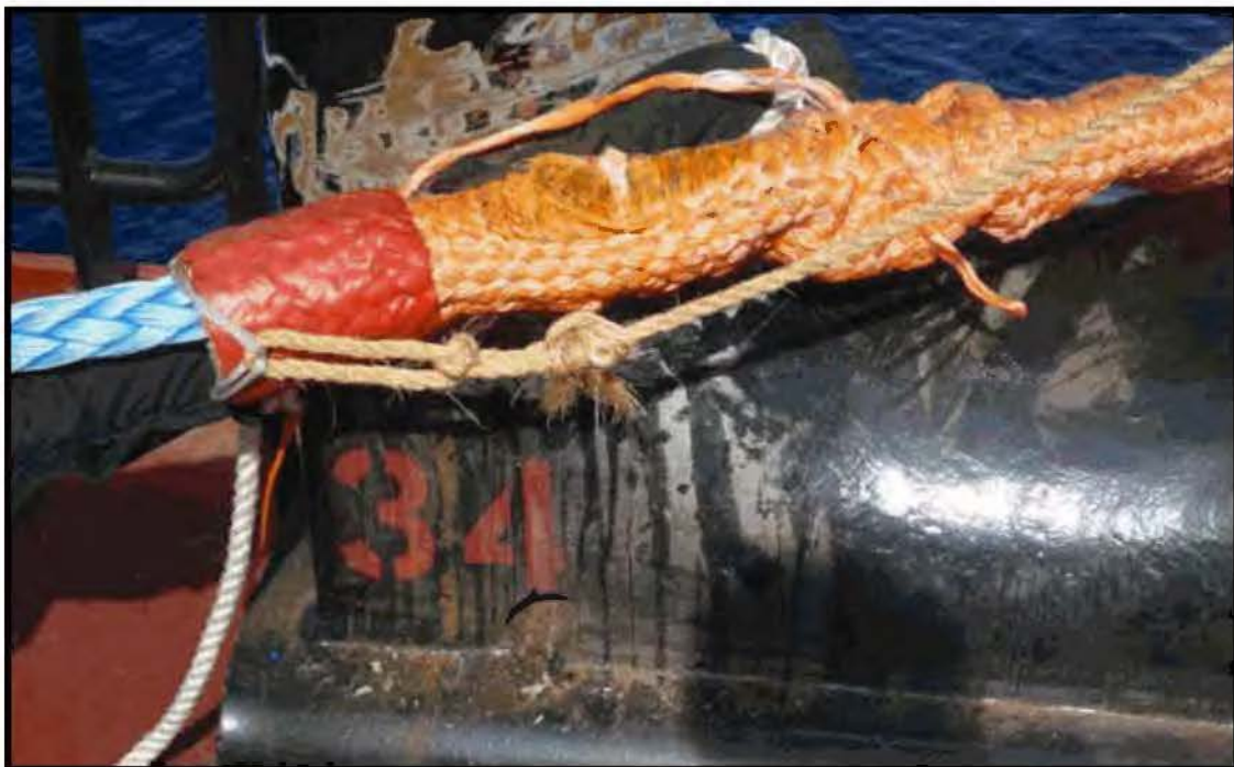
Figure 4-4. Mooring Line Damage
