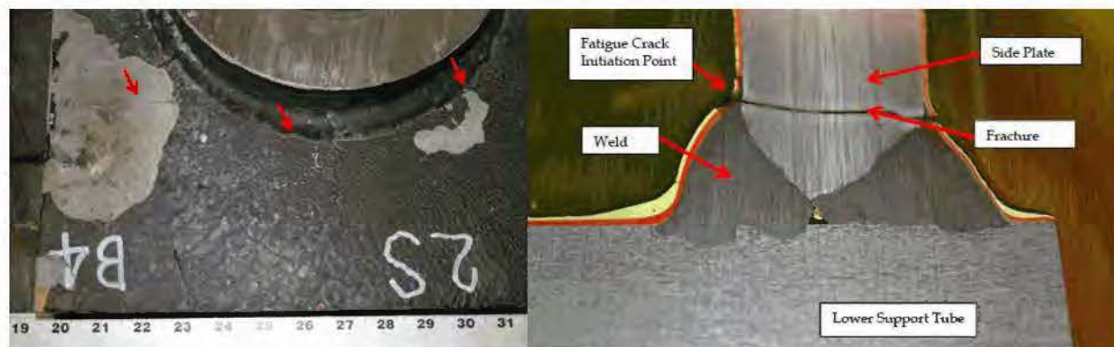
Figure 15. Details of Weld and a Crack Initiation Point
