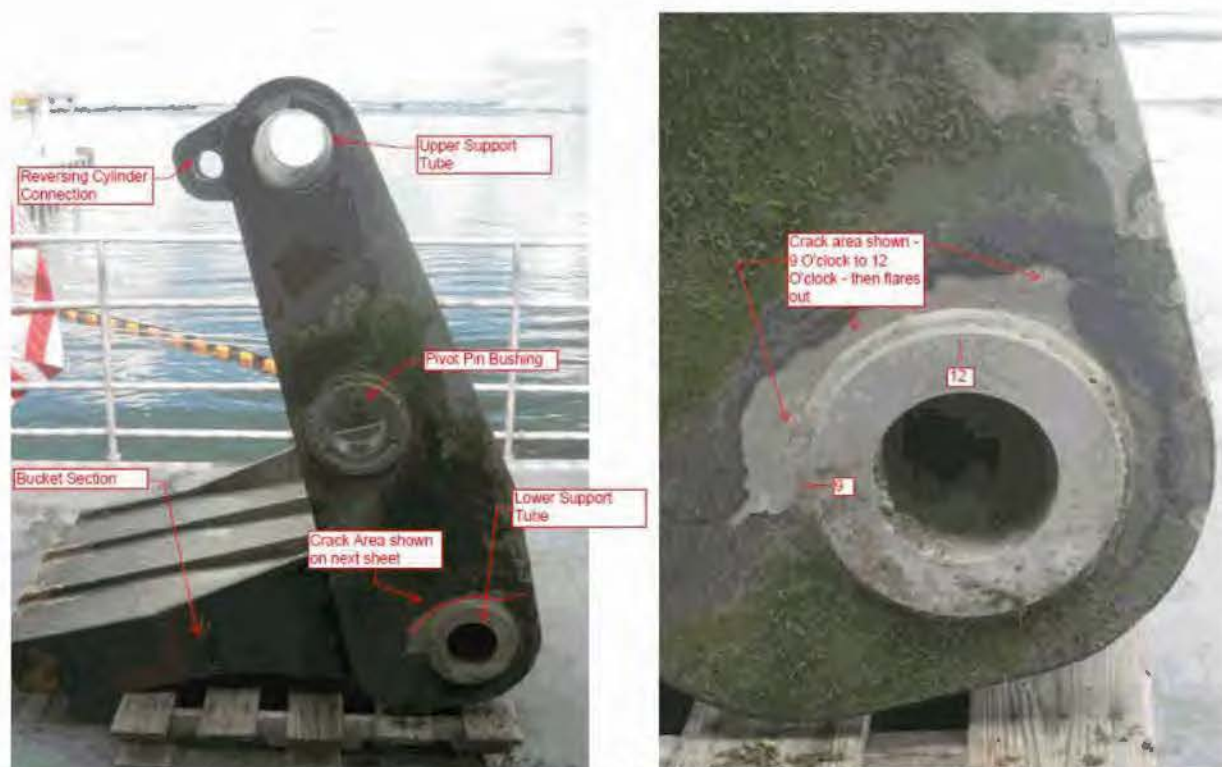
Figure 14. USNS Spearhead Port Waterjet Reversing Plate showing Fatigue Crack
