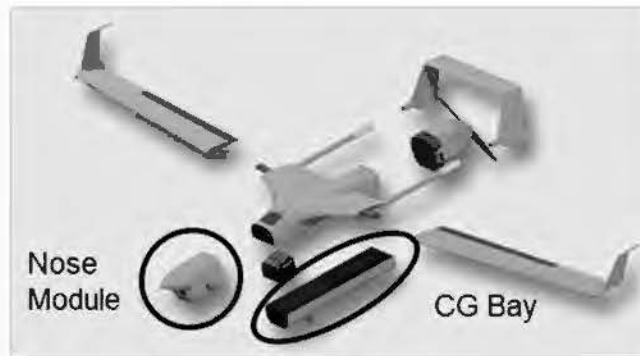
Figure 3-4. Air Vehicle Payload Modules
