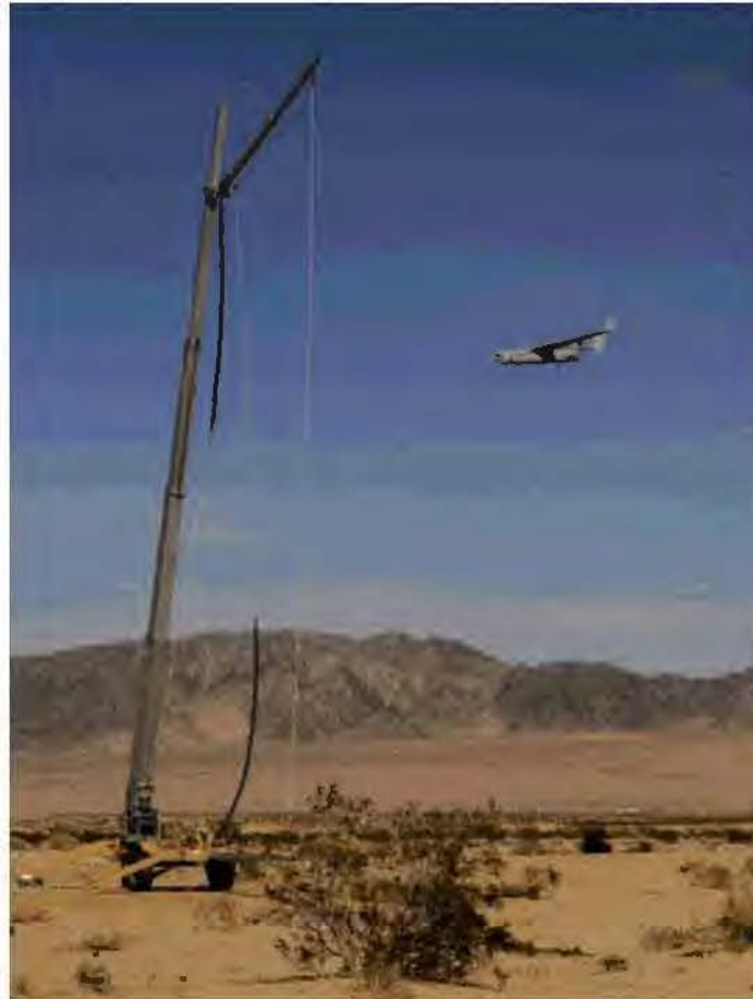
Figure 1-6. RQ-21A Recovery System
